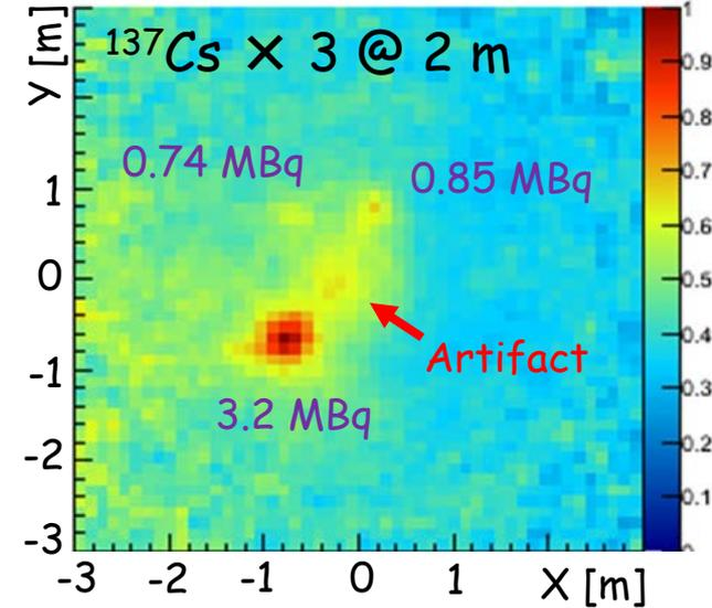
Electron tracks provide 4 times better S/N than usual Compton imaging!
