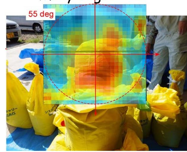
$^{137}\text{Cs}$  cal-source @ 50 cm ( $0.36 \mu\text{Sy/h}$ )
